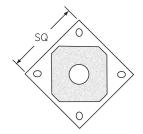
1C5 diamond pattern slotted base plate prestressed to pole
